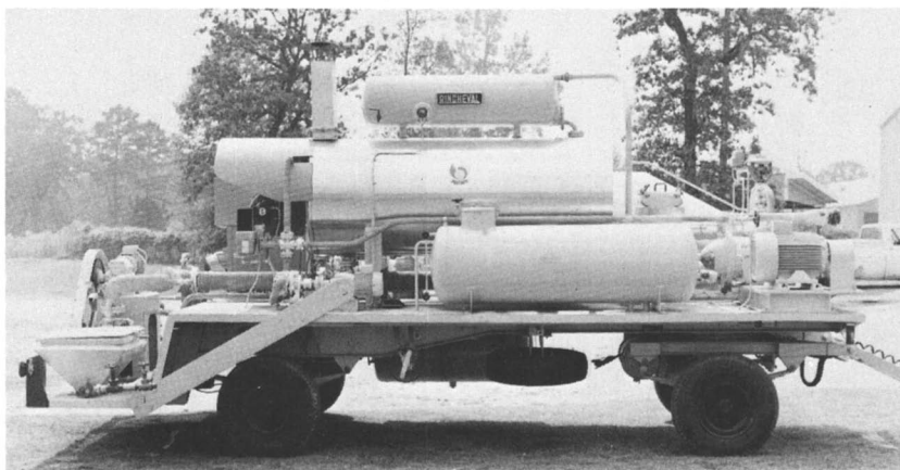
Figure 2. SNPA's mobile sulfur and asphalt blending equipment
