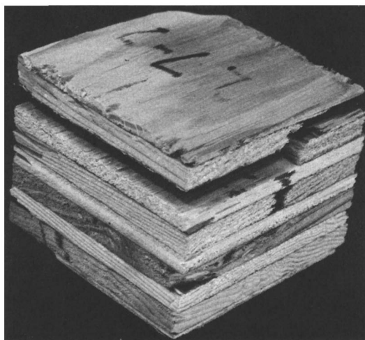
Figure 1. Typical fracture of sulfur-bonded plywood sample, tested according to ASTM D-1037-72a. The failure occurred at 134 psi.
