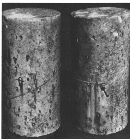
Figure 9. Photograph of sulfur-infiltrated concrete cylinders immersed 10 months in distilled water. Note the abundance of flowery sulfur extrusions and the trace of a sulfur-filled fracture (↖) formed during demolding. Dark rings are iron sulfide.
