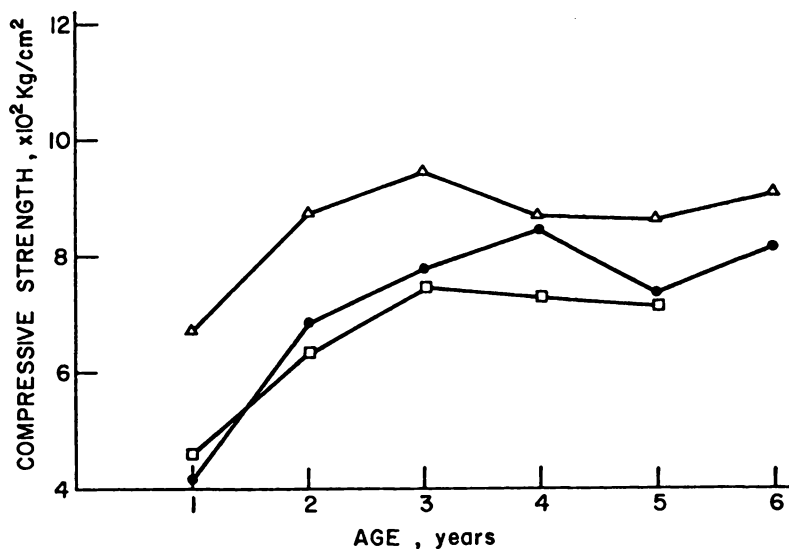
Figure 1. Effect of age on compressive strength of bamboo culm. (●) Meng-tsung bamboo, (Δ) Makino bamboo, (□) thorny bamboo.
